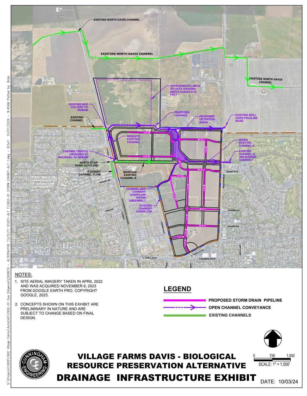
The development of the project includes a new conveyance channel and a centralized storm water detention basin which provide storm water detention to mitigate for the increase in peak flow from the development and provides storage mitigating for the increased runoff volume.
